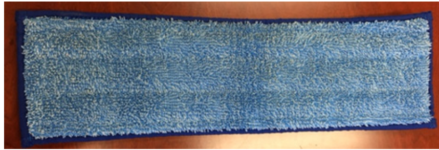
Sample B: Note the nonuniform discoloration of backing
