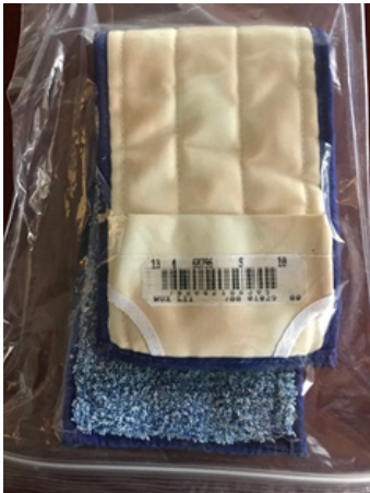
Sample B: Note the nonuniform discoloration of backing
