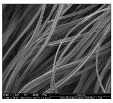
Figure 4: Scanning electron micrograph – new unlaundered microfibre flat mop (mag.=1000x)
